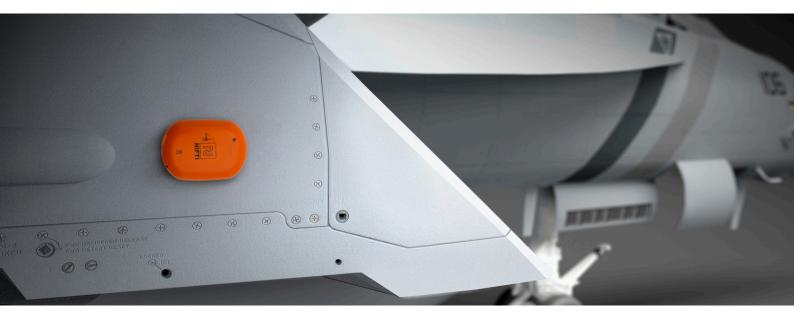
NIFTI<sup>™</sup> is the Non-Intrusive Flight Test Instrumentation system that revolutionises aircraft flight testing by enabling rapid, affordable and flexible flight trials.
