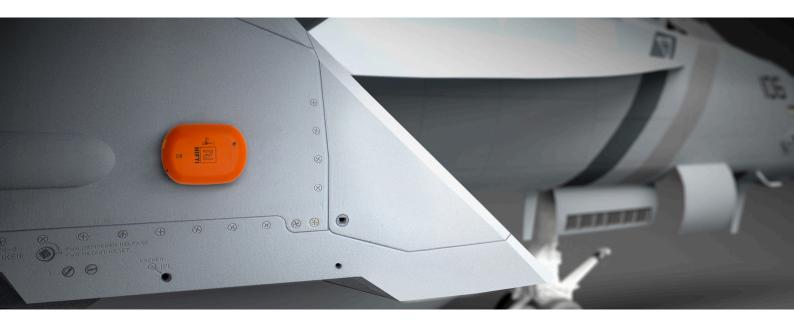
NIFTI™ is the Non-Intrusive Flight Test Instrumentation system that revolutionises aircraft flight testing by enabling rapid, affordable and flexible flight trials.
