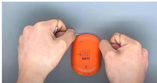
Figure 9: Sawing motion through Mounting Pad using NIFTI Removal Tool.
