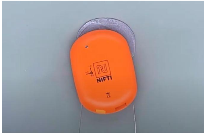
Figure 10: NIFTI Removal Tool sawing through the adhesive
