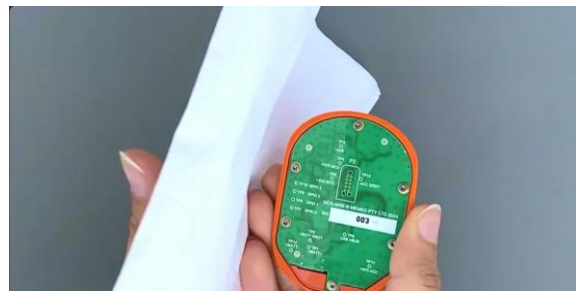
Figure 2: Cleaning back of Sensor Node with cloth and solution.
