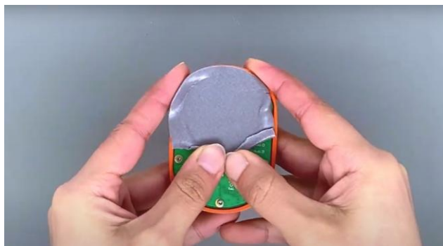
Figure 11: Removal of Mounting Pad from back of NIFTI Sensor Node.
