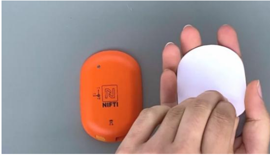
Figure 3: Remove white backing from the Mounting Pad.
