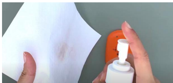
Figure 12: Final clean of Sensor Node using 50% IPA and distilled water solution.
