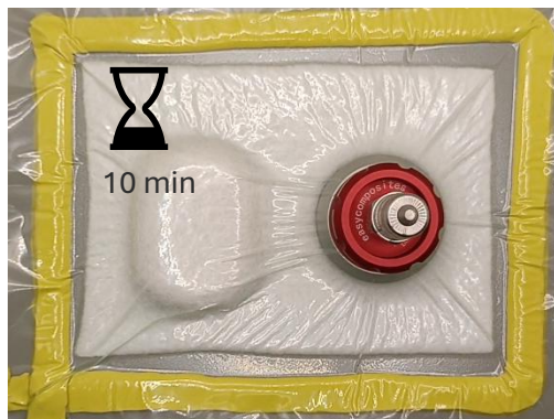
Figure 11 10: Maintaining seal for 10 minutes.
