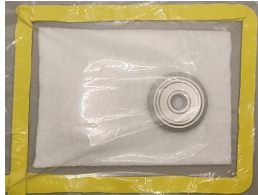
Figure 6: Vacuum bagging film fixed in place by sealant tape.
