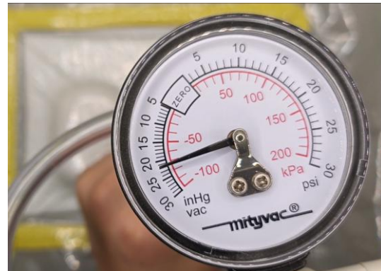
Figure 10: pressure gauge showing at least 66 kPa.
