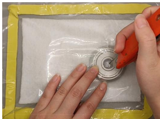
Figure 77: Piercing hole over valve base plate.
