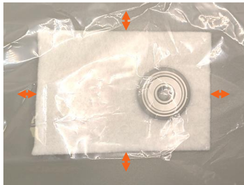
Figure 3: Vacuum bagging film covering application area.
