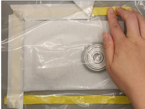
Figure 5: Sealant tape backing removal starting at one end and working around.
