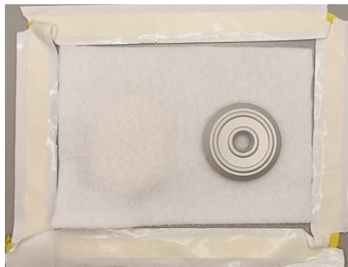
Figure 4: Sealant tape applied to surface around breather cloth.
