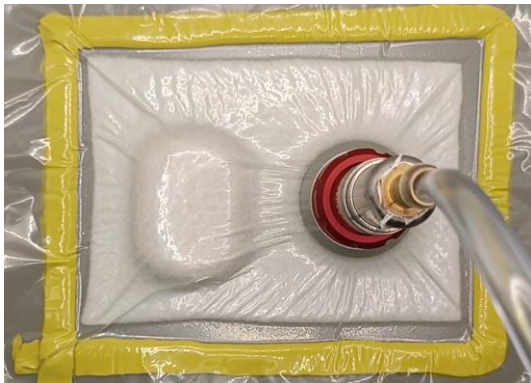
Figure 9 9: Applying pressure to vacuum bagging.
