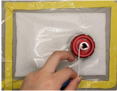
Figure 88: Attachment of vacuum valve to base plate and Teflon tape.
